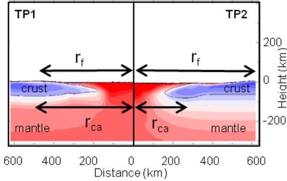
**Figure 2:** Final basin form for two impacts with the same energy (80 km diameter impactor, 15 km/s velocity) into targets with different thermal profiles (TP). TP1 and TP2 both have a crustal thermal gradient of 10 K/km. In the mantle, temperatures are initially at the solidus in TP1, but are sub-solidus in TP2.  $r_f$  is final basin rim radius,  $r_{ca}$  is crustal annulus radius.
