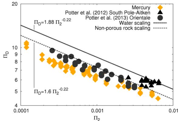
**Figure 3:**  $\Pi_D$  as a function of  $\Pi_2$ .  $\Pi_D$  is a crater size measure defined as  $D_{ic}/(M_i / \rho_i)^{1/3}$ .  $\Pi_2$  is a gravity-scaled impact size defined as  $3.22 g r_i / u^2$ .  $D_{ic}$ : transient crater diameter;  $M_i$ : impactor mass;  $\rho_i$ : target density;  $g$ : surface gravity;  $r_i$ : impactor radius;  $u$ : impact velocity. Scaling laws from [17].
