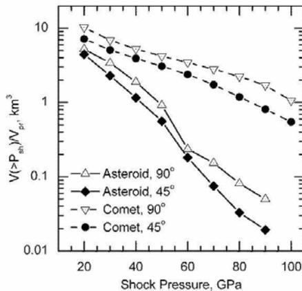
**Figure 1:** Volume of target subject to shock pressures above a given value normalized to projectile volume for asteroidal and cometary impacts and different impact angles (45°, 90°) on a mixed cell target (case C).
