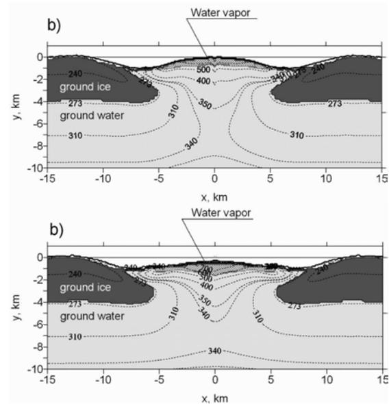
**Figure 2:** Isotherms and phase state of pore water (relative to local temperatures and pressures) below a Martian crater with rim diameter of ~30 km formed by an asteroid (upper) and a comet (lower) impact. Ice: dark gray; water: light gray. Regions of water vapor stability are cross-hatched. Lithostatic pressure increases the boiling point. Consequently, liquid water may exist at a temperature up to the critical point (650 K) below the central peak.
