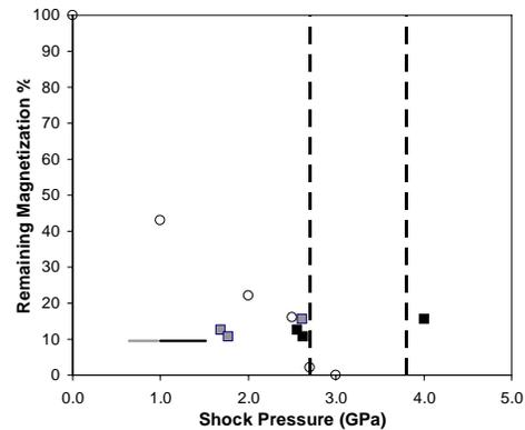
**Figure 1:** Demagnetization of pyrrhotite: black symbols – principal stress (squares – single shock, line – double shock); grey symbols – pressure assuming elastic shock; open circles – static experiments [9]; dashed lines – phase change region in pyrrhotite from shock data [11].
