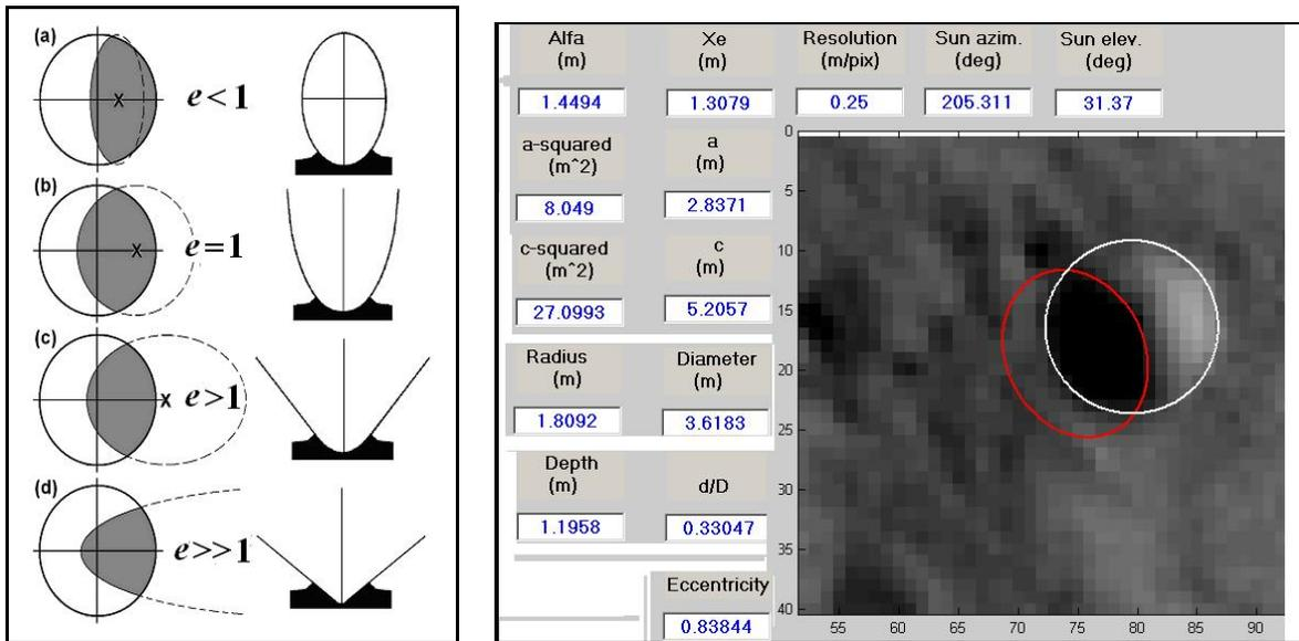
**Fig.1** - Crater shapes (right) and their associated shadows (left). From top to bottom: (a) elliptical (b) parabolic (c) hyperbolic and (d) conical craters. Corresponding eccentricity values are also given. All four of the measurable craters (Fig. 3) correspond to (1a). **Fig.2** - An example of the output from a shadow measurement trial, this one taken from crater (see Fig.3, below). The effects of "pixillation", which sets the resolution limit on the shadow method, are evident in the image.
