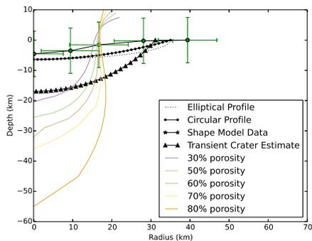
Figure 2: Crater profiles from Monel-Monel porosity study. Higher target porosity resulted in greater crater depths, while crater diameters were less affected by target porosity than crater depths.
