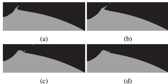
Figure 1: Images from the  $\text{SiO}_2$ -Monel simulation showing the eventual overturned flap: (a) ejected material follows expected trajectory out of crater; (b) hinge forms during crater excavation; (c) material collapses at hinge; (d) flap of hinged ejected material has overturned.
