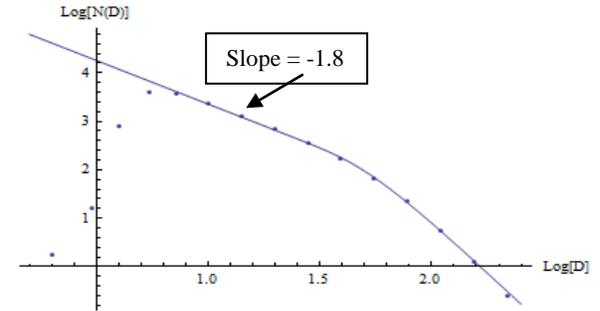
Figure 3: Log-Log Plot of number of craters per bin,  $N(D)$  vs  $D(km)$ , based on Barlow's Mars catalog, and the curve from the model in Eqs. (5) to (8). Data for  $D < \sim 8km$  is undercounted.
